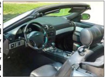
Gray. One of the options on my car is the Select Shift Transmission which is a dual gate console shifter which allows you to shift the transmission as a manual, similar to today's cars paddle shifters. As this option was not on a lot of the cars mine became 1 of 79 built. Not exactly 1 of 1 but still pretty cool!"
